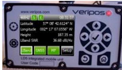
All LD5 variants supplied incorporate an **L-Band module** to receive Veripos corrections. (A1 variant is a demodulator only)
